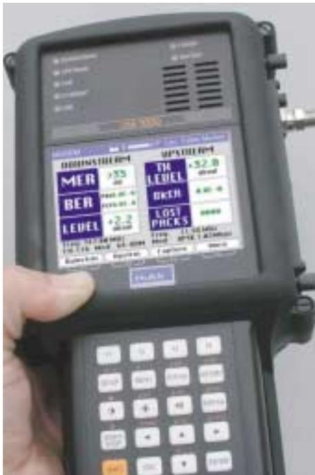
Since cable modems are capable of transmitting over a wide dynamic range (+8 to +58 dBmV), adding attenuation in the reverse path causing the modem to transmit at the upper range of its power level minimizes ingress from the home. Assuming the desired power level at the CMTS is 0 dBmV, 48 dB of attenuation in the reverse path is an appropriate target. Still providing ten dB of headroom for plant variations due to changes over time and temperature.
