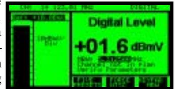
ratio is reduced one dB for each dB the carrier level is lowered, but improves the distortion performance, critical to good BER performance, on Digital signals is improved by 2 dB for every dB change in analog signal level. Note that for the total power level, the sum of all carriers, to remain the same (maximum allowed to not over modulate the laser), the video carrier levels will be set a little low to allow the digital levels to be set higher.
