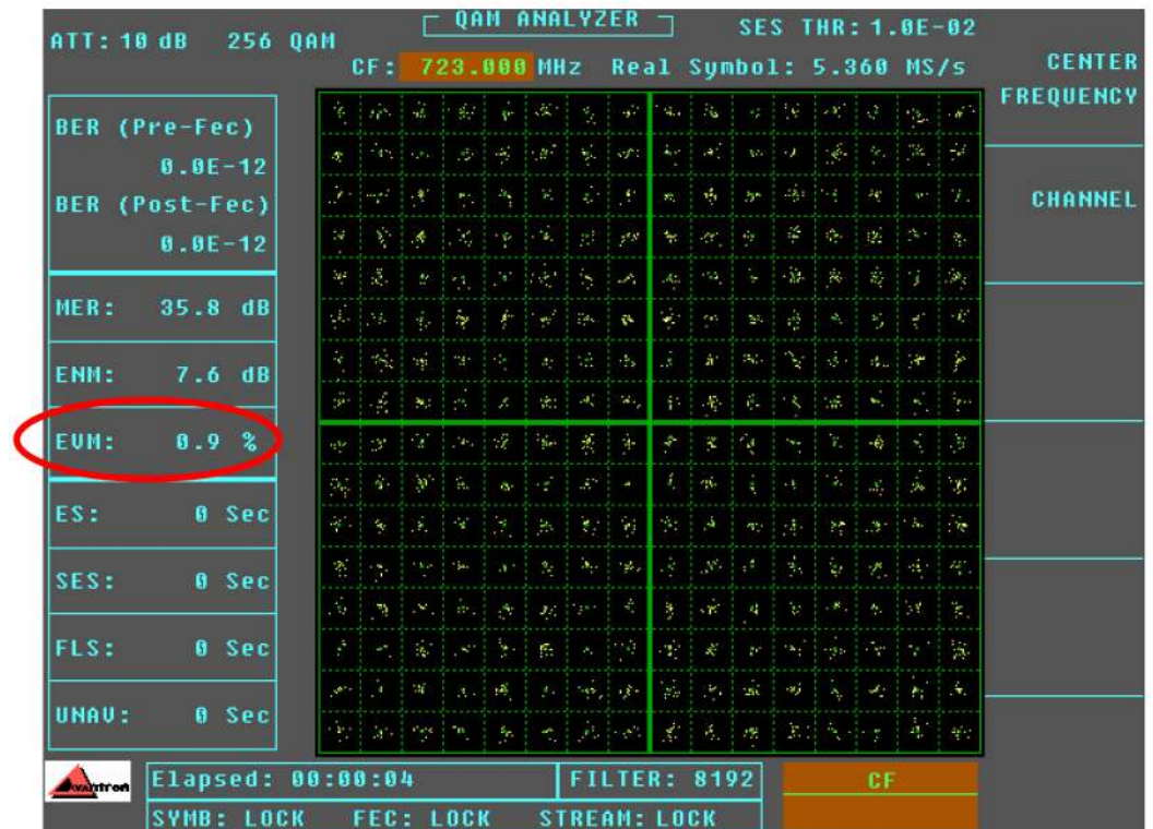
Figure 16. The EVM of This Downstream 256-QAM Digitally Modulated Signal Is 0.9 Percent. (Courtesy of Sunrise Telecom)
